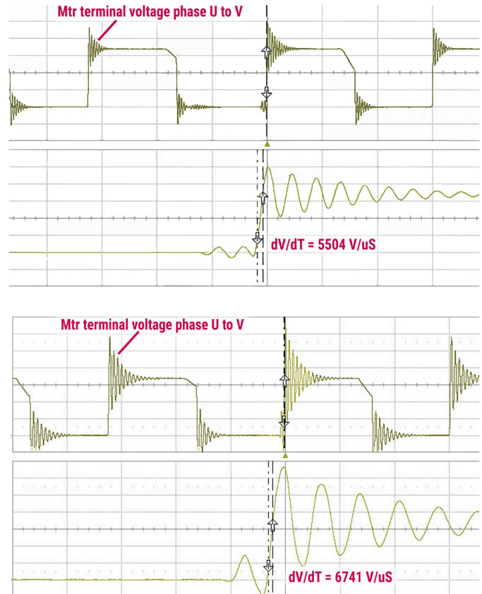
Figure 11: No choke, 25-ft leads. Peak motor voltage = 988 V
