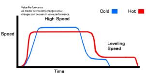
Temperature (heat) in a hydraulic elevator system is primarily built when oil is being recirculated through the control valve back to the tank. Therefore, the majority of the heat is generated during the up leveling of the elevator. There are many factors that will affect the time spent in leveling, such as slow-down distance and up-transition adjustment, with the most overlooked factor being the minimum oil temperature.
