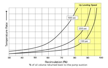
system pressure is low (<100 psi) with a fast contract speed of 150-plus ft/min, extending the distance to 6 in. for 25 ft/min may be necessary. Verifying the slow-down distance on install, prior to valve adjustment, is an important factor for minimizing leveling distance to help manage temperature swings. Keep in mind that most controllers will default to 6 in. for every 25 ft/ min and should be shortened to 2 in. for every 10 ft/min when possible.
