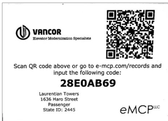
Figure 6: eMCP tag mainline disconnect or controller (MCP, 2023B)
