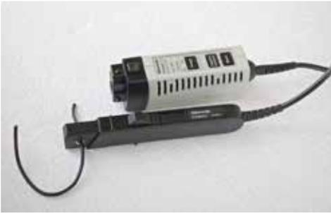
Current probe, designed to be used with an oscilloscope. For small, out-of-range current, the conductor can be wrapped two or more turns through the jaws, multiplying the effect.
