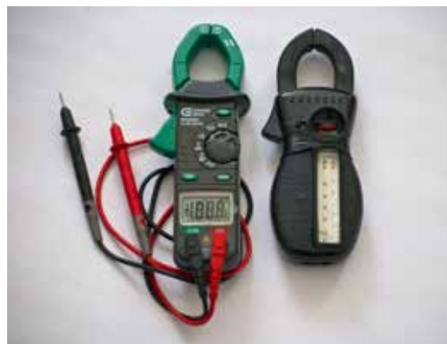
Digital and analog clamp-on ammeters. Either one works.
