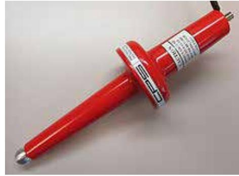
High voltage probe for up to 50 kV. The barrier at the center of the probe body isolates the user's hand from the live object under test. The probe tip is a corona ball, which protects the user against corona discharge and arcing by distributing the electric field gradient. The user should stand on an insulated dry rubber mat to limit grounding and wear high-voltage gloves (available at Amazon), if possible, for redundant protection.
