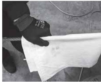
Method for checking for lubrication
