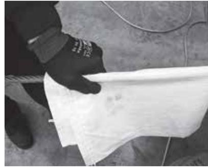
Method for checking for lubrication
