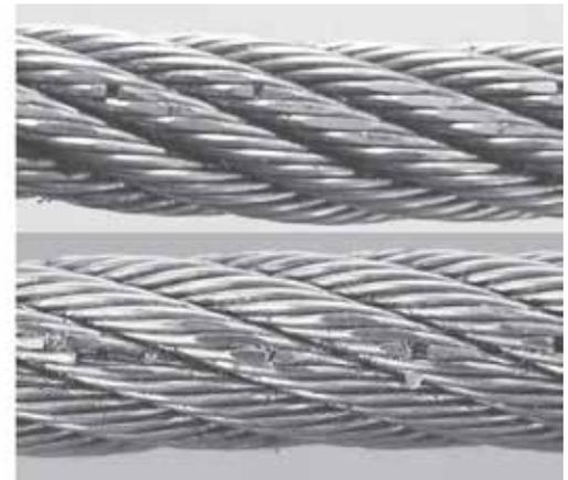
Figure 10: Wear zones in ropes with fiber cores (8x19S-NFC) and ropes with steel core (8x19S-IWRC)
