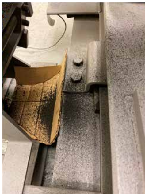
Figure 1: Example of metal particles under a pinch point
