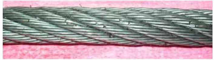
Figure 5: Count the number of distributed (crown) wire breaks within a rope “lay length.” Up to 32 are permitted in normal wear conditions; only 16 are permitted in unfavorable wear conditions.
