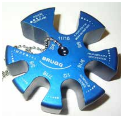
Figure 1: A rope go/no-go gauge is suitable for checking rope diameter.
