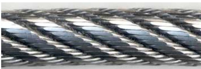
Figure 4: Very clear crown wear, the main effect of which is reduction in rope diameter.
