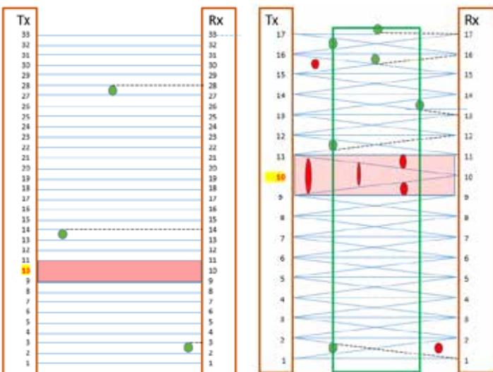
Figure 8: Failure of one optical element (emitter or detector)
