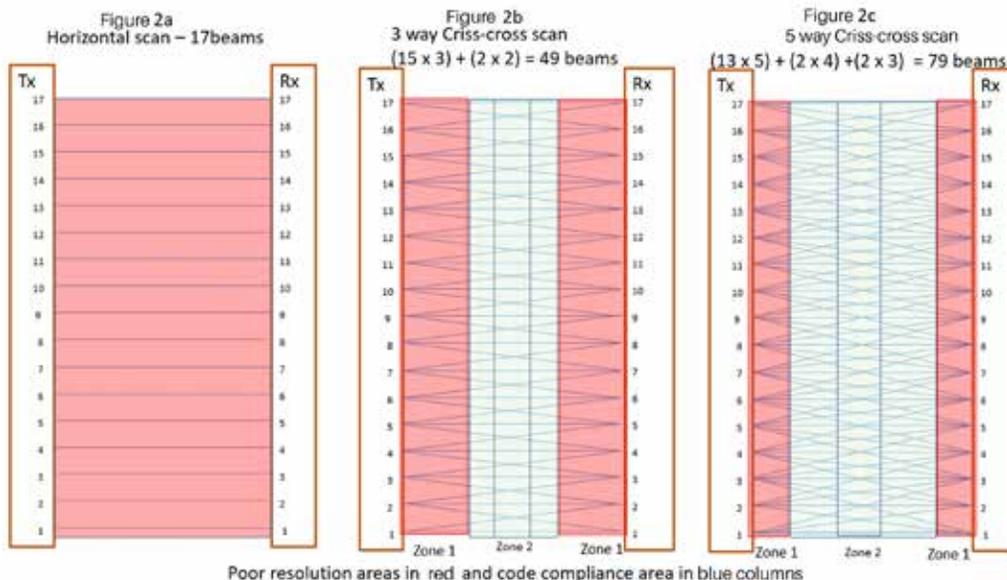
Figure 2: Crisscross arrangement for a light curtain with 17 emitter/detector pairs.
