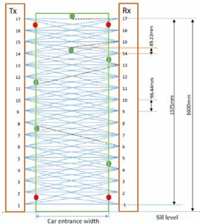
Figure 6: Light curtain with five-way crisscross scanning arrangements: Tx = vertical array of emitters; Rx = vertical array of detectors; green dot = 50-mm object/obstruction detected; red dot = 50-mm object/obstruction undetected; and dashed line = obstructed beam path.
