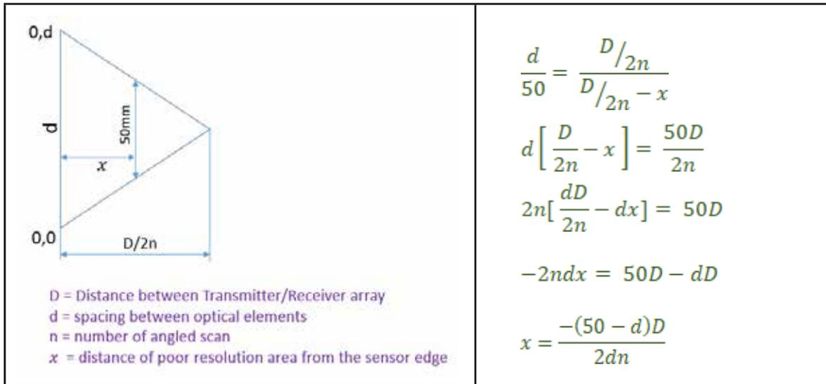
Figure 4: Distance x is the width of the poor-resolution area from the sensor edge: note that, per the code, the protective devices shall be capable of detecting an obstacle of at least 50 mm in diameter. However, only the vertical distance of 50 mm (which is a safer assumption) is considered.
