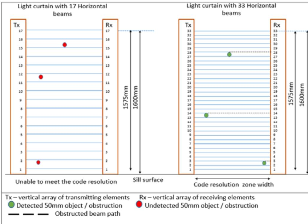
Figure 1: Light curtain with horizontal beam arrangements
