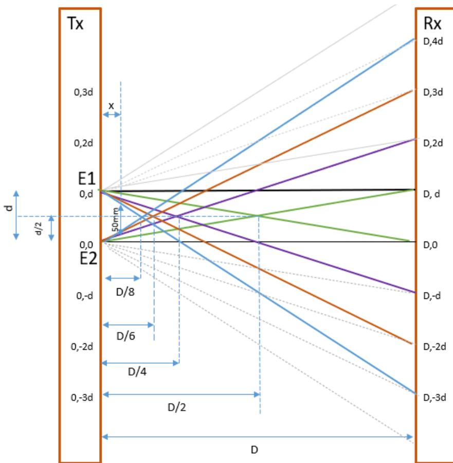
Figure 3: The arrangement of detectors scanning two emitters in a nine-way-scan system (four angled-up, four angled-down and one horizontal scan):  $d$  = spacing between the consecutive emitter/detector;  $D$  = spacing between Tx and Rx arrays
