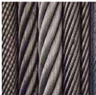
Figure 5: Right-handed and ordinary (or regular) lay rope
