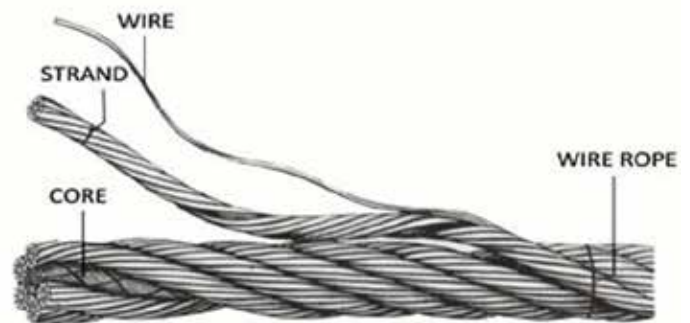
Figure 2: Structure of a standard rope
