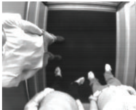
Figure 1: ESPROS/VOL images showing different levels of elevator cab volume consumption (l-r): 15% full; 50% full; 75% full
