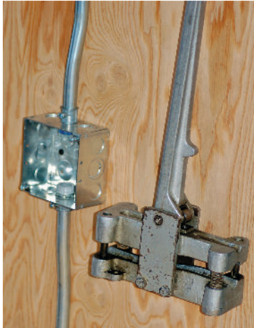
Figure 1: An offset bender makes both bends simultaneously where metal raceway enters a box.
