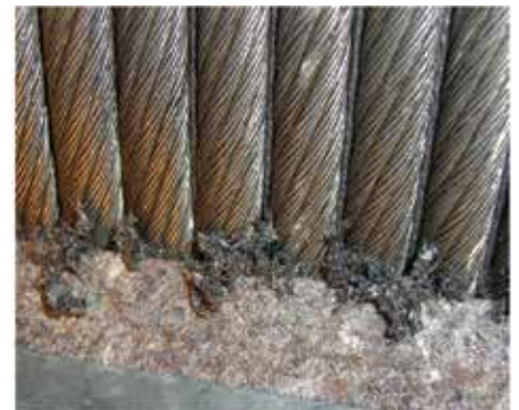
Figure 8: A case in which an automatic rope lubricator is placed too close, and the felt touches the ropes.
