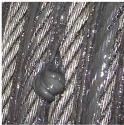
Figure 6: Solvents are a major component in many spray-lubricant cans and are incompatible with the original lubricant applied by the manufacturer. Results are in the photo at right, in which the original rope lubricant has deteriorated due to the effects of a solvent and is being squeezed out of the rope core. The end result of this interaction is the deposit of a slimy coating on the rope surface.
