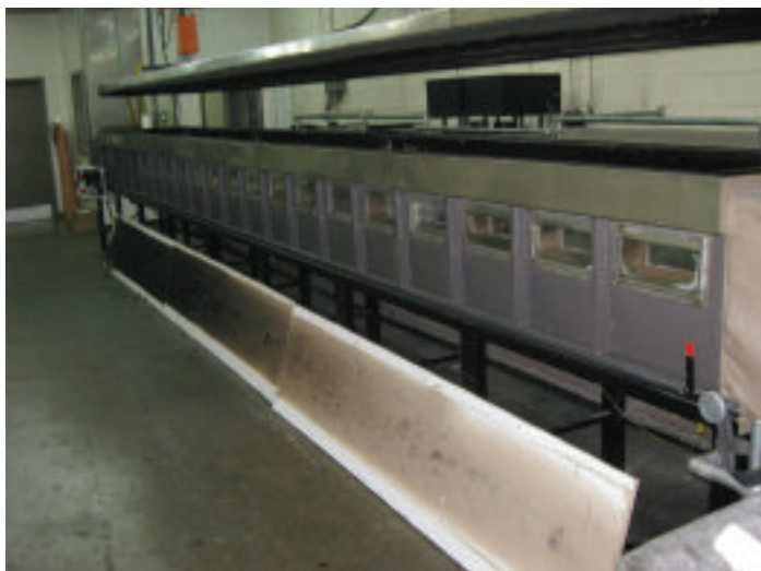
Figure 1: A Steiner Tunnel
