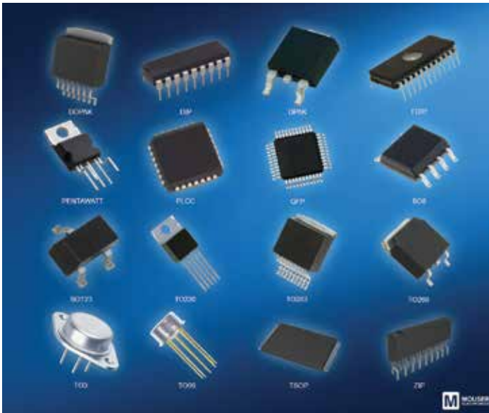
Figure 1: ICs come in numerous packages with standardized pin spacings. They can be mounted on a circuit board or inserted into IC sockets (graphic courtesy of Mouser Electronics).
