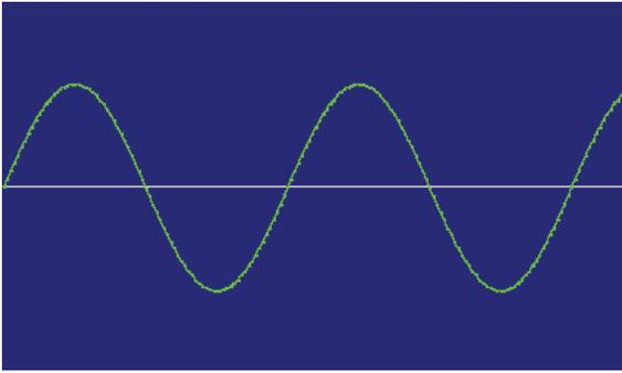
The induction motor thrives on an analog sine wave or a digital rendering that closely approximates it.
